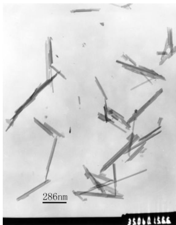
Figure 3 The TEM image of the bare ATP nanoneedles.
